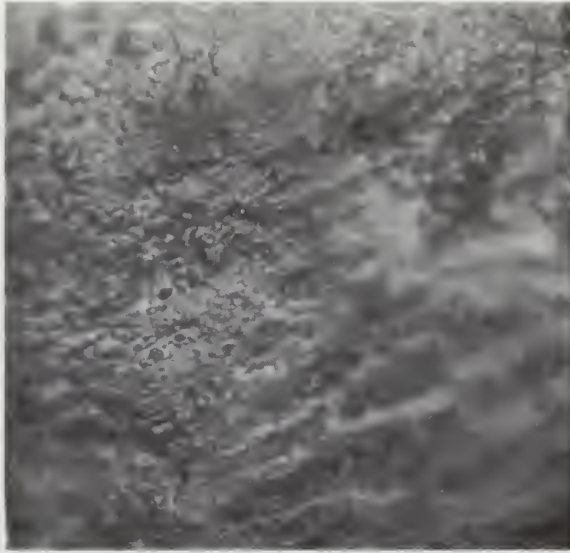
FIGURE 24. BIAxIAL TENSILE SPECIMEN YIELD SURFACE; EPON 828 + 10 pph CTBN R-151 (LARGE PARTICLES). (450X).
